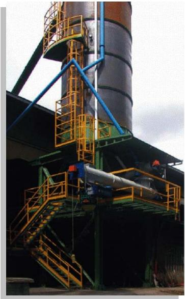
The silo has a weighing system installed under the storage bin.
