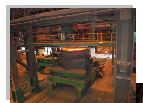
Double powder covering system with 50 cubic meters capacity storage bin and two rotating powder distributors.
