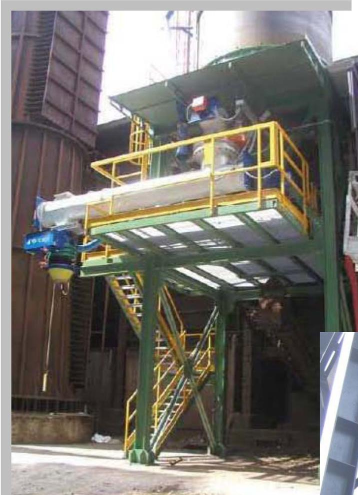
Alternative solution of the existing filter dust handling system.
