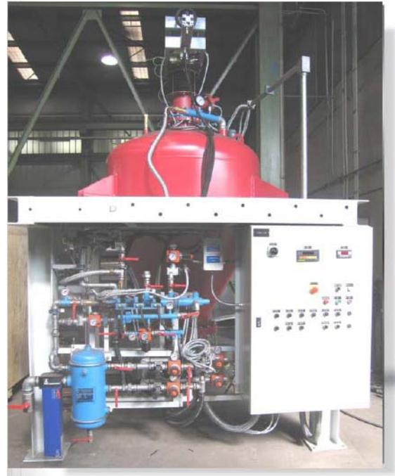
**Steel work plant installed automatic system for coal storage, pneumatic conveying and injection in electric arc furnace**
