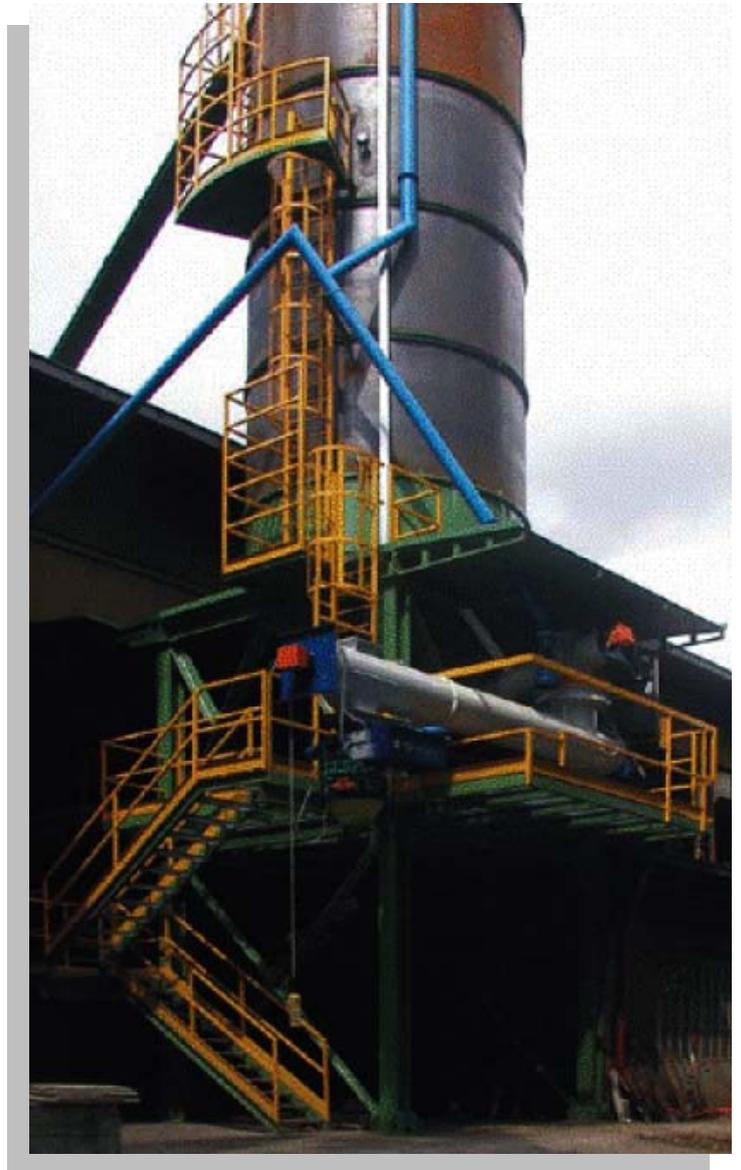
The silo has a weighing system installed under the storage bin.
