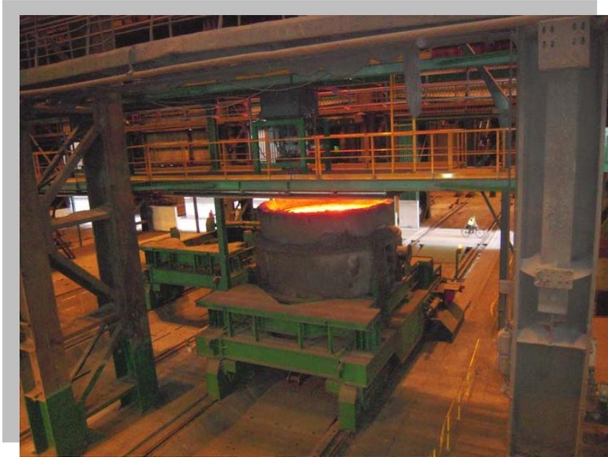
**Double powder covering system with 50 cubic meters capacity storage bin and two rotating powder distributors.**
